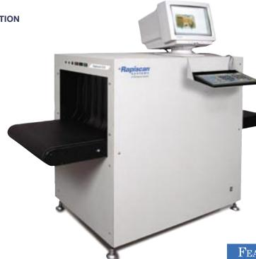
The **Rapiscan 515** is a dual energy, compact X-ray system for space restricted installations. Dual energy imaging provides automatic color coding of materials with different atomic numbers so that screeners can easily identify objects within the parcel. The system is equipped with a removable control panel to facilitate mobility.
